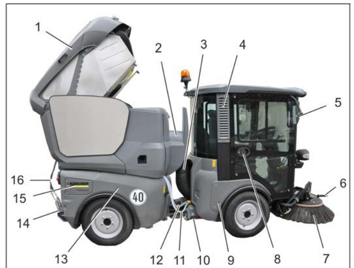
Figure: MC 130 with raised waste container (driver's side)
